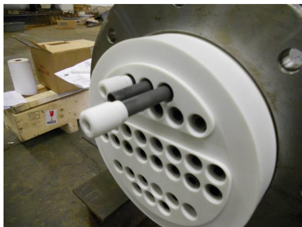
Teflon tubesheet with tube nut on tube
