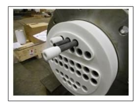
Gaining access to the tubes is quick and convenient making process side cleaning or a clogged tube replacement simple, safe, and economical. The ceramic's extreme hardness and inherent low adhesion properties make hydro-blasting effective without worry of damaging the tubes.
