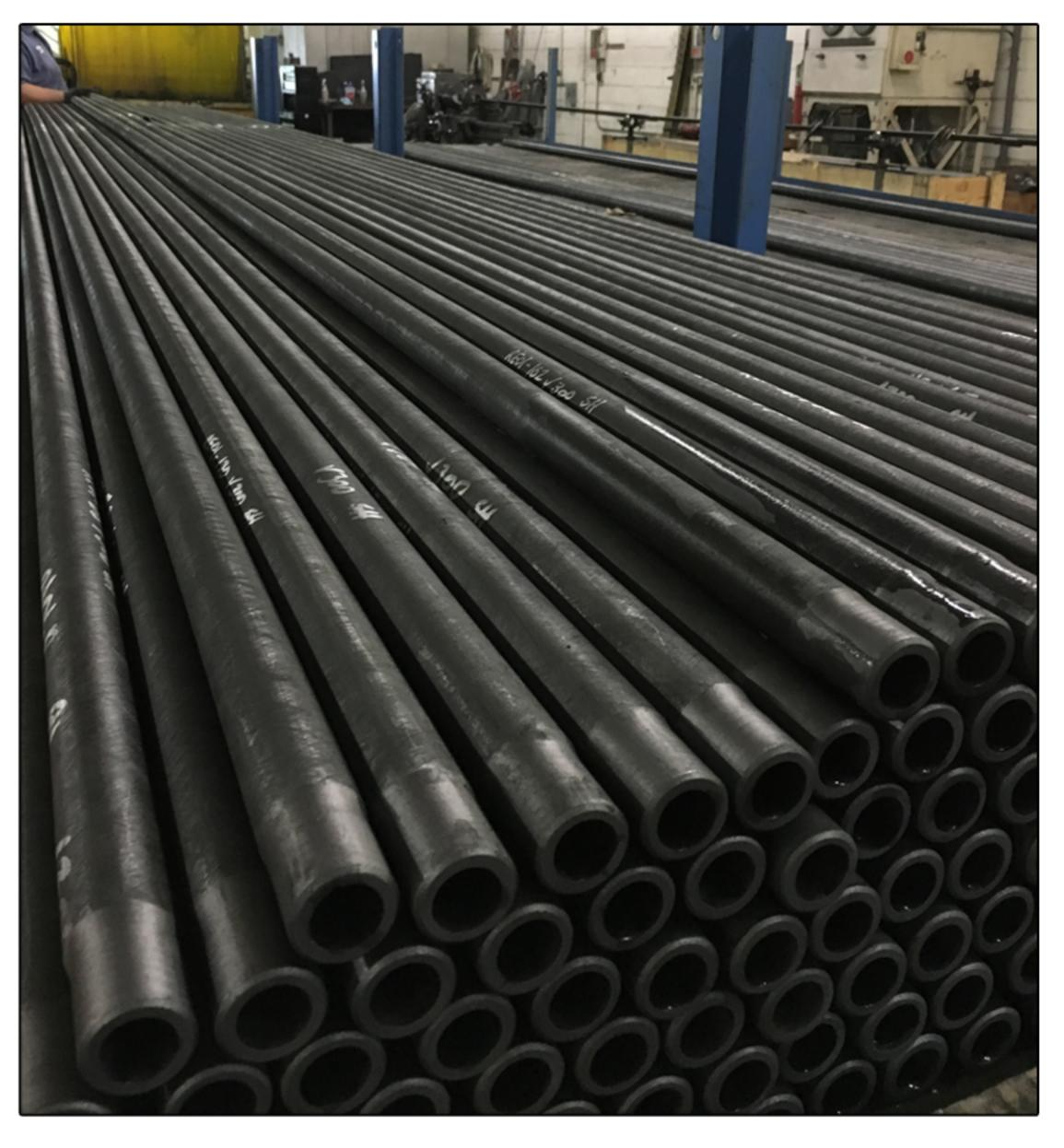
This process will be done multiple times, controlling the pore size within the graphite. Baking the mixture at this temperature will transform the binder and furan resin into carbon. At this point, the tube material is carbon-graphite.
