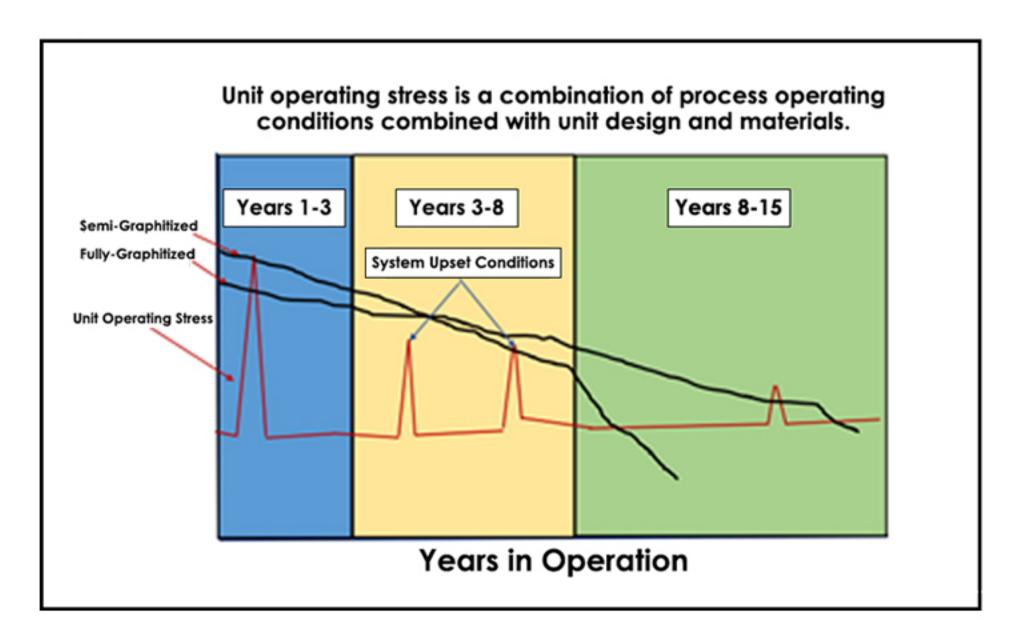
Raw graphite material is impregnated with phenolic resin to make it impervious. But equally important, impregnation greatly increases the strength of the graphite material. As the unit ages the resin continues to cross link and eventually will start pulling away from the graphite base on a microscopic level, resulting in lower tube strength. At the same time, the tubes experience random microcracking imparted by slight vibration associated with cycling or
