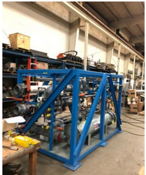
The Impervite® graphite condenser offers thermal efficiency and 100% corrosion resistance. The compact and modular design allow all of the components to be stored in standard shipping containers during transit and when not in use. A uniquely designed process automation arrangement addressed the process challenges, including the highly variable feed composition and the need for quick switching capabilities between parallel systems.
