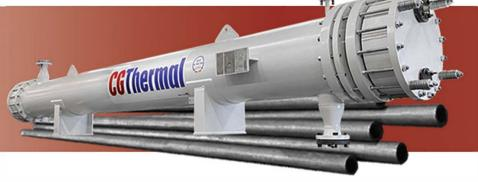
CG Thermal Impervite® impervious graphite tube is manufactured by subjecting a fully araphitized porous graphite tube to our state-of-the-art proprietary vacuum/temperature/pressure impregnation of modified phenolic resin.
